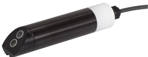
The TTurb is a digital sensor for optical turbidity measurements according to the 90° IR scattered light method. Depending on the sensor it can be used in pure water up to 100 FNU as well as in raw-, waste- and process waters up to 1000 FNU. TTurb is available with a 10 m or a 2 m fixed cable.
