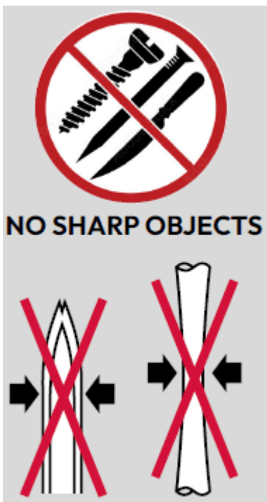
Figure 4 - Installation: No sharp Objects. Do not pinch the cable.
